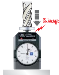
Large dial gauge, LED lamp and sound ease operation. TOOL MASTER
